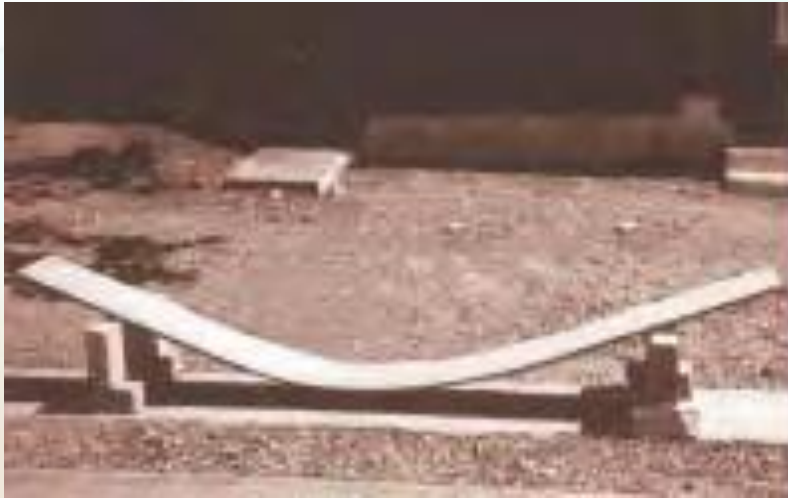
Ferrocement plank 3000 x 300 x 25 mm, bends like a bow when supported as shown above
